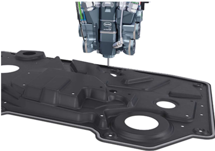
The fully automatic dosing application according to FIPFG technology is carried out with the CNC-controlled MK 825 PRO precision mixing head and the DM502 dosing system with high dosing accuracy.
