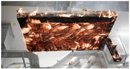
In the fire protection simulator at ETH Zurich, Henkel's new LOCTITE HB XE adhesive was able to demonstrate its excellent fire protection capabilities.
