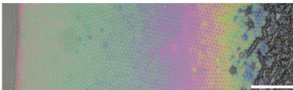
Figure 1. Microgel monolayer drying on a hydrophobic substrate. The monolayer is drying towards the left side, where the meniscus is visible. Scale bar = 10 \mu m.
