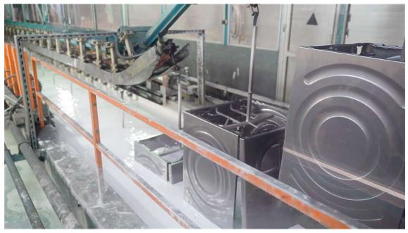
Cleaning and coating steps give metal surfaces important properties such as corrosion protection and paint adhesion, thus making a key contribution to quality and performance in subsequent application.
