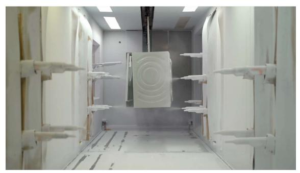
The Cleaner & Coater technology enables users in the metal industry to reduce the number of process steps in their metal pretreatment by half while also saving energy and water.
