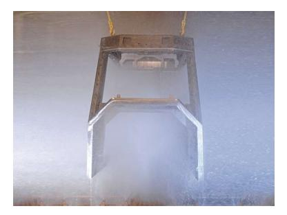
Henkel cleaning and metal pretreatment innovations can enable low-temperature cleaning to operate at 38°C instead of 60°C achieving significant energy reduction.
