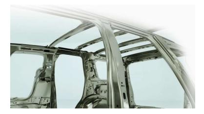
Henkel structural adhesives to replace welding, such as in cabin assembly, can enable lightweighting, reduced material consumption and a carbon footprint reduction up to 15%.
