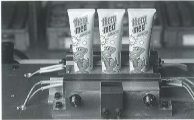
Station for testing the seal on toothpaste tubes and the cardboard supports. Inside the retail outlet, the tubes must be tamper proof.
