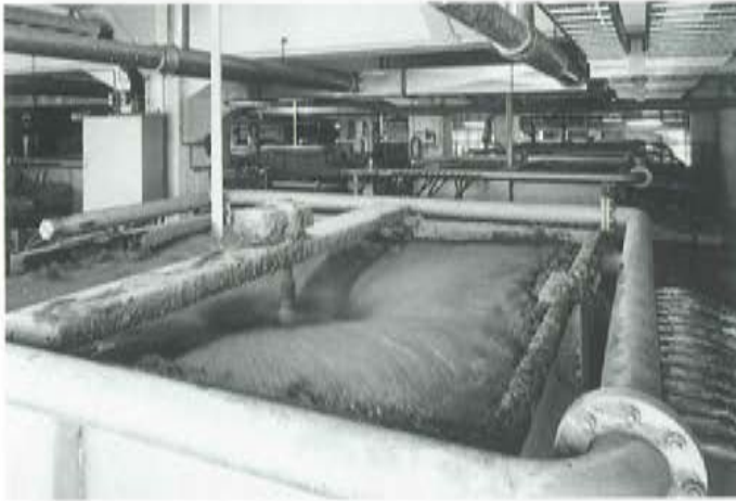
Flotation processes in a paper mill: printing inks are removed during the recycling of wastepaper.
