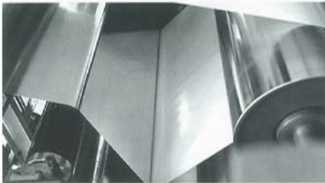
Trend to water-based film and foil laminating adhesives: production of composite film with solvent-free film adhesives.
