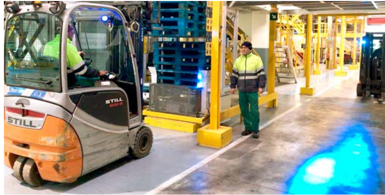
Areas where employees and forklifts work side-by-side pose a collision risk. Thanks to a modern radio system, forklift drivers are alerted if employees are detected within a range of one up to 6.5 meters. This helps avoid collisions.
