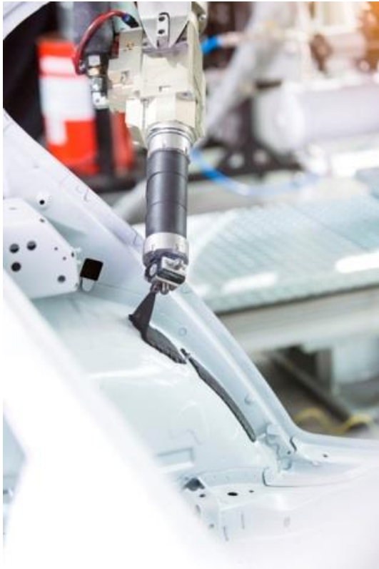
Weight-saving, clean and efficient: Automated application of LASD compounds in the paint shop. (Photo: Henkel, PR015)
