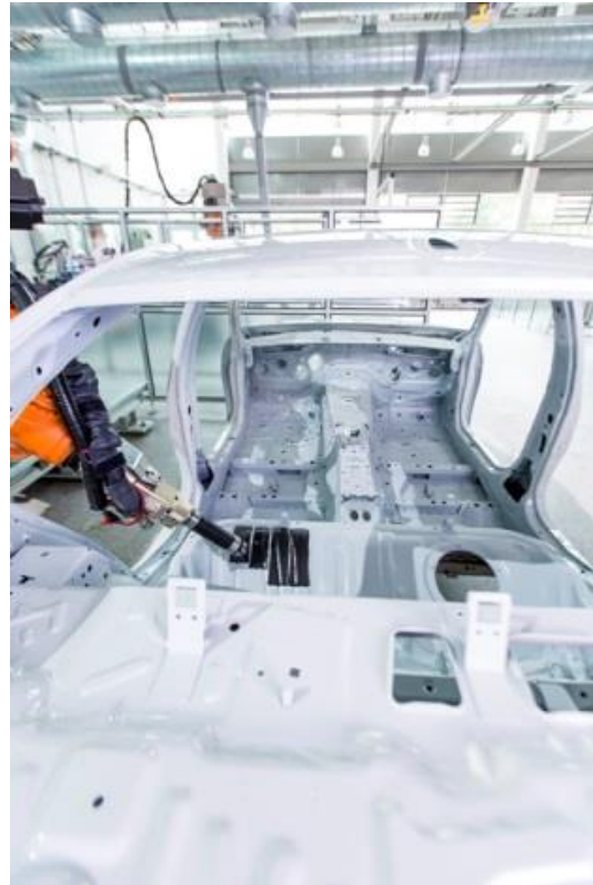
New, innovative liquid-applied sound deadeners for the automobile industry. (Photo: Henkel, PR015)
