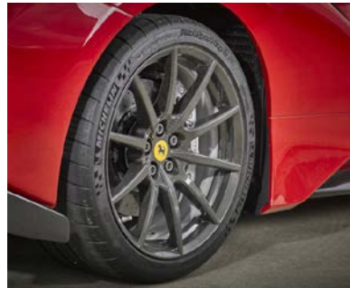
Henkel and Carbon Revolution have joined forces to speed up the development of lightweight wheels that are made from a single piece of carbon fiber.
