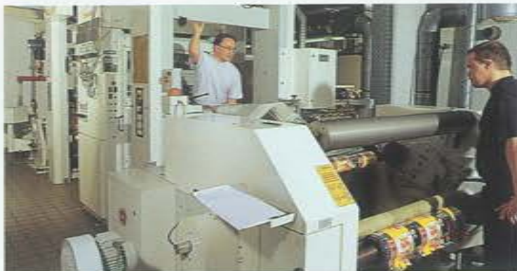
Solvent-free laminating adhesives. Henkel tests the adhesion of multi-layer films and foils in its Düsseldorf pilot plant.
