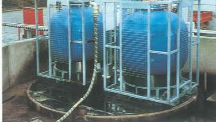
Henkel Ireland now sells its former production wastes as recoverable material. Organic impurities are removed from aqueous aluminum salt solutions for this purpose.
