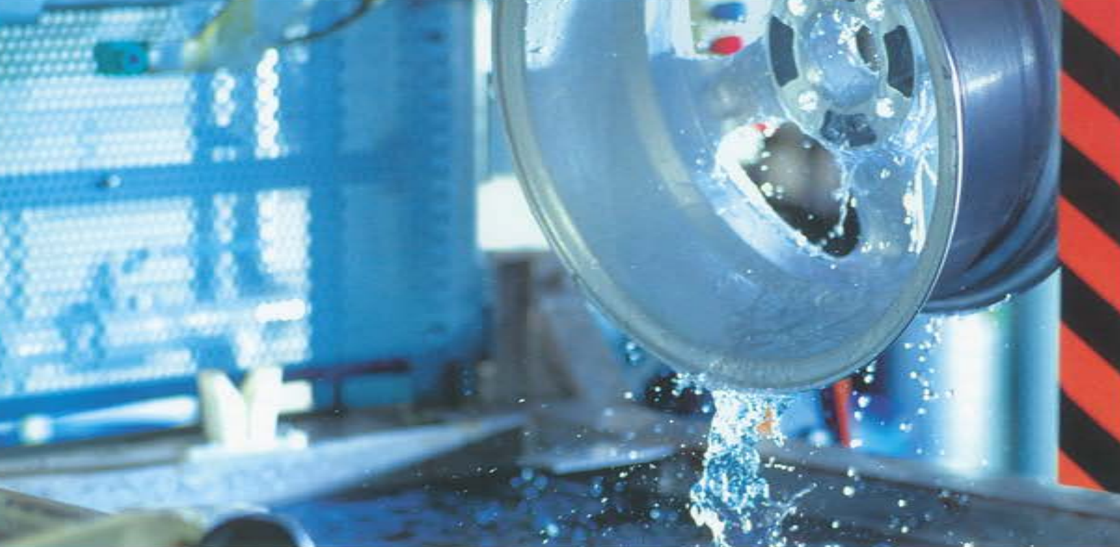
Environmentally compatible corrosion protection – an aluminum wheel rim being treated in a chrome-free dipping bath.
